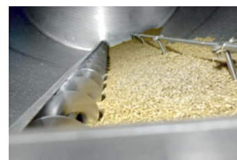
The section containing the discharge spiral rotates continuously, functioning like a shovel
