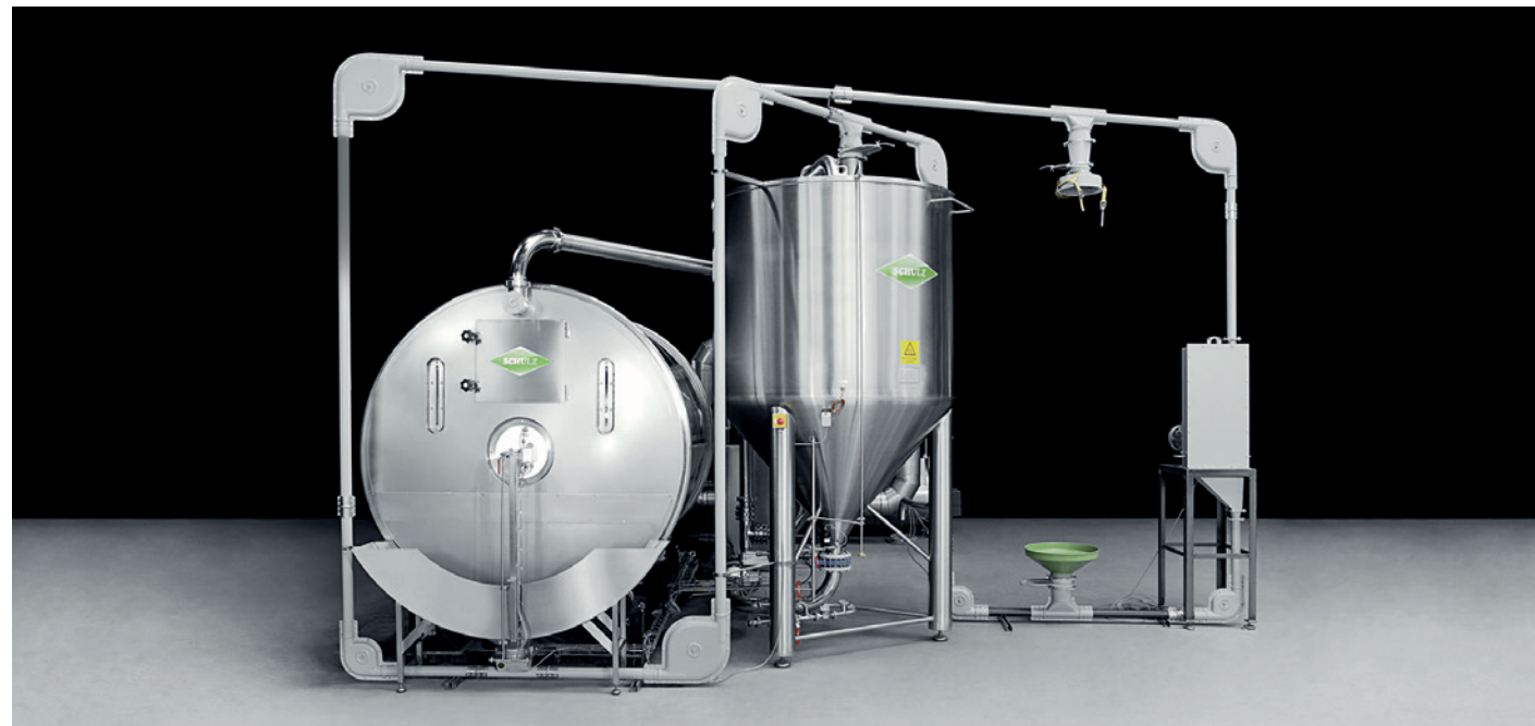
Insulated drum with an external rotary drive for germination and kilning operation without requiring green malt to be transferred. Malt which has been thoroughly mixed and dispersed ensures consistently excellent quality.
