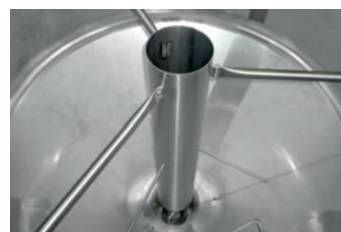
The central circulating pipe ensures aeration and circulation in the steep tank
