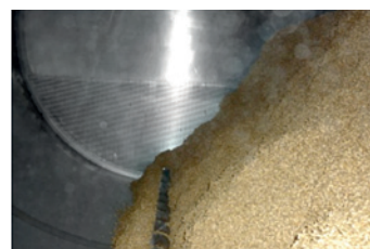
After being loosened up by the rotating motion, the material is discharged
