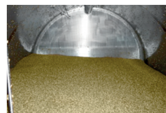
A rotating drum allows intensive mixing and uniform distribution
