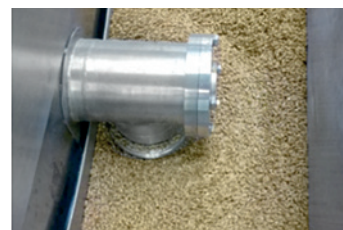
Drum is emptied via a permanently fitted screw running in the opposite direction of the casting
